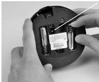
Look for blinking communications light.
